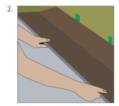
Next, draw a line to mark out the perimeter of the laid plank and then set the planks aside.
