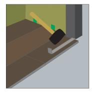
After the groove ledge has been trimmed, place the board in place and tighten with a pull bar. The installer must be sure that the required expansion gap has been maintained and the flooring is not pinched.
