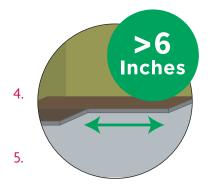
Maintain proper spacing (at least 6" for planks, and equal to half its length for tiles) between end joints for best appearance.
