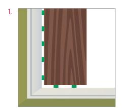
Starting from the left with the tongue-side facing the wall, carefully place the first board in place, using spacers to leave a ¼" expansion gap between the wall and edges of the plank or tile.
